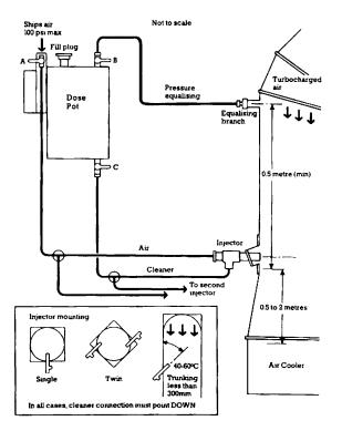
**NOTE:** Always consult the engine manufacturer before installing the injectors.
